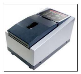
SuperShakIR is a Grinder mixer which produce fine powder. It is able to crush the sample, KBr Chunk, powder and mixing them for making the transparency pellet. It can also make fine powder from solid sample because of capability of high power grind. Fine powder is good for measurement in ATR method and it is possible in this device.
